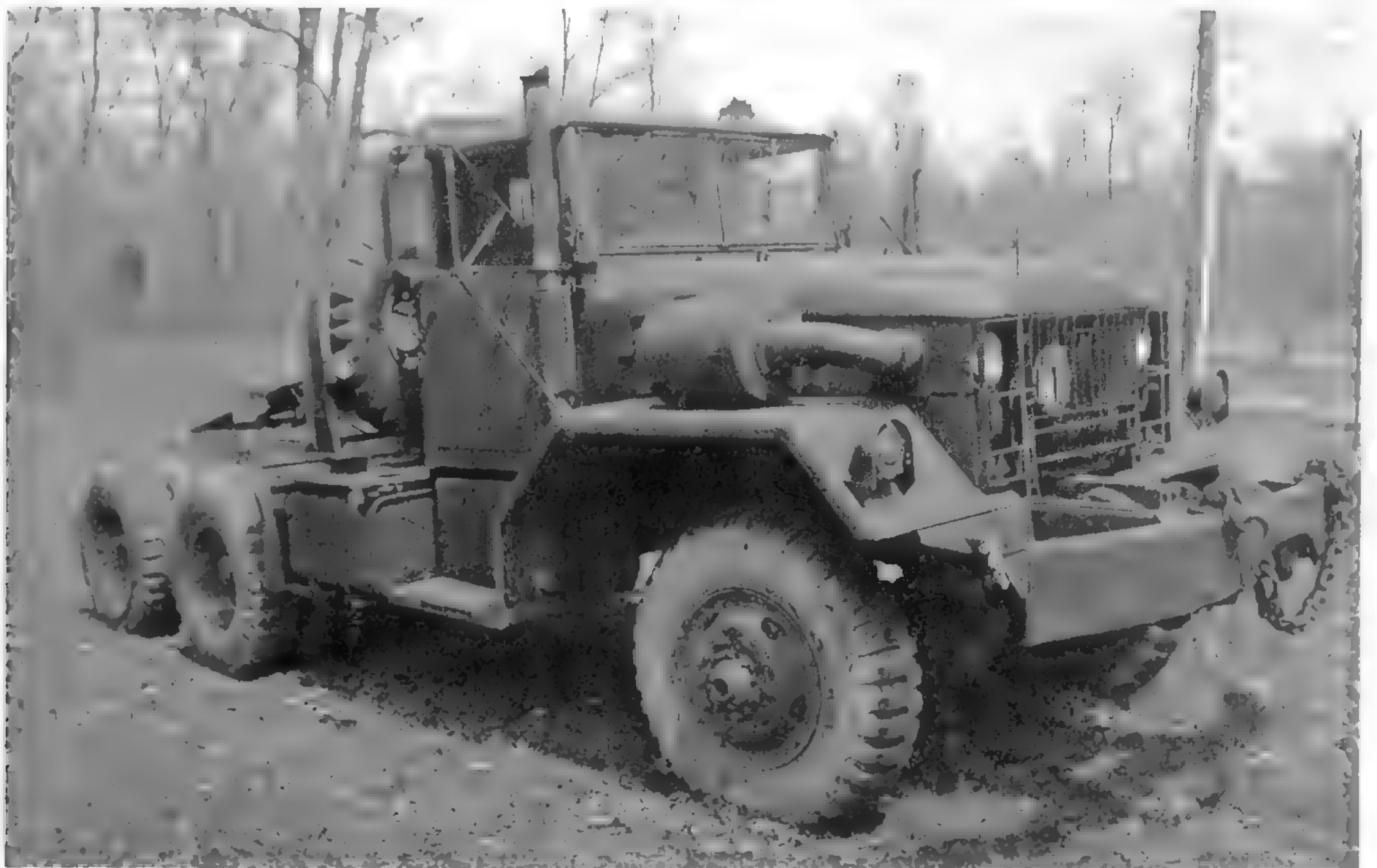
This M52A1 with winch is a Diamond T product. It is one of a group of trucks that were re-powered with the Mack ENDT-673 engine in the early 1960s. (Photo courtesy of TacticalTruck.com)
